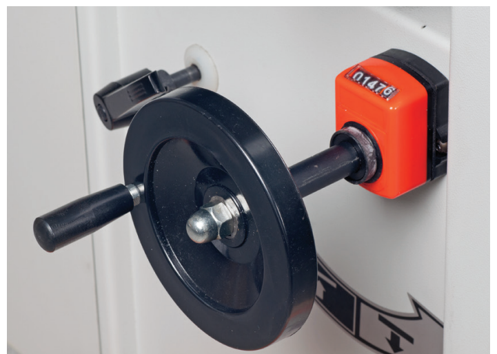
Thickening table rise and fall control wheel
