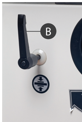
Rise and fall clamping handle (A), in the locked position clamping handle (B), in the un-locked position
