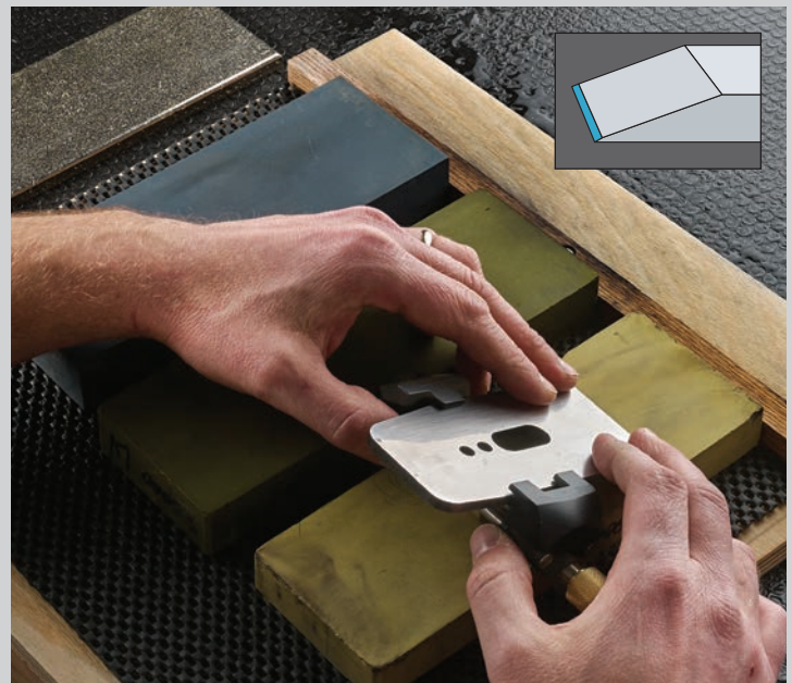
4. Polishing the cutting edge on an extra-fine stone prepares the edge for fine woodworking.
