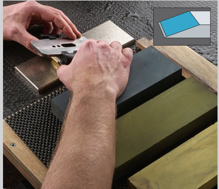
2. A coarse diamond plate will quickly shape a bevel, followed by a medium stone to remove the scratches left by the diamond plate.
