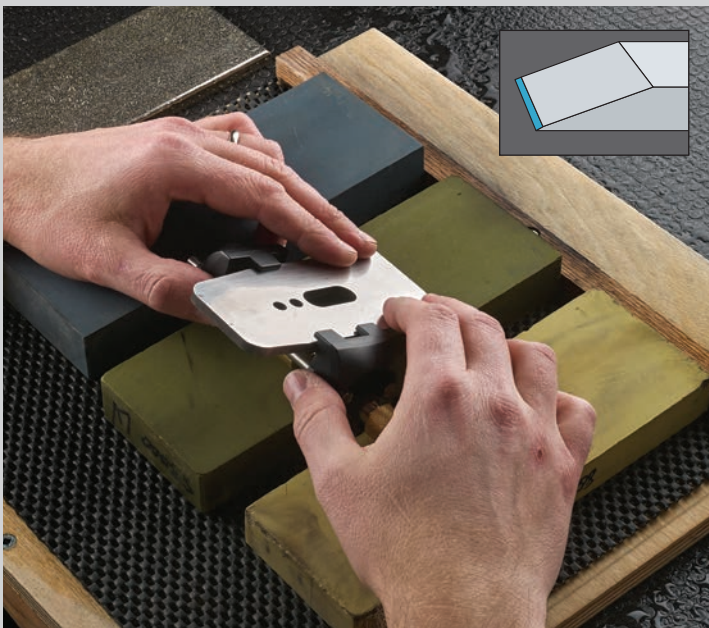
3. Honing the cutting edge on a fine stone prepares it for general use or refines the edge for polishing.
