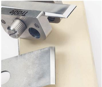
The final honing is a very precise process and great care should be taken when adding the secondary bevel as the 5° differential in angles is a very small difference. The secondary bevel will work even if it is very small. It doesn't need to be much more than 1.0mm in width for it to achieve the desired effect. Remember, if you want to touch up the tool, this bevel can be elongated a number of times so, always keep the grind down to an absolute minimum.
