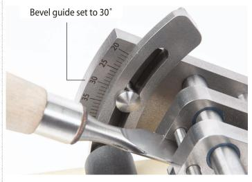
Select the given angle and tighten the guide securely placing the guide and the tool on to a suitable abrasive such as a 6000g or 8000g water stone. Make sure the stones have been flattened to ensure no unevenness. With plenty of water on the abrasive, simply pull the guide and tool towards you applying gentle, but even pressure to the blade on the stone.
