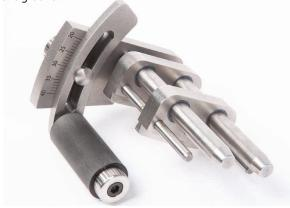
The guide has two bars on to which the honing guide is placed. The guide can be positioned anywhere along the bars for use. The setting of the micro-bevel guide relies upon a 25mm projection from the guide just as it is used on the machine. If the tool is to be touched up, you should project the tool precisely to 25mm and tighten the tool in the guide.
