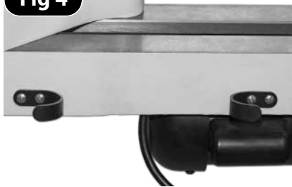
Steel hooks in position
