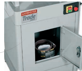
Robust, welded steel stand with storage cupboard
