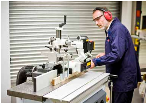
Sliding table fitted with mitre fence and work clamp for precision work
