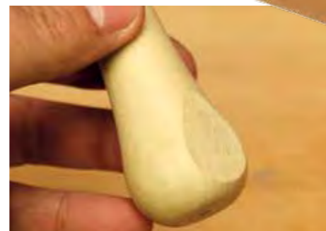
The butt chisels have a small flat on the underside of the handle...
