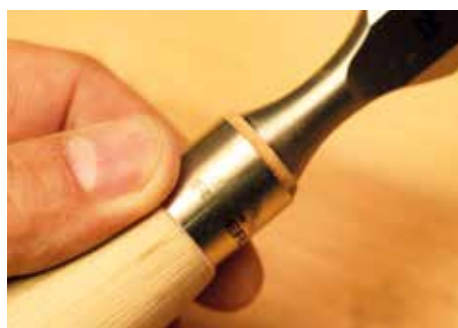
The leather washer and stainless ferrule is common across both styles of chisel
